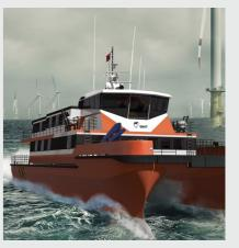
BMT designed the 36m Service Accommodation Transfer Vessel (SATV) for the Formosa 1 Offshore Wind Farm, in Taiwan.
