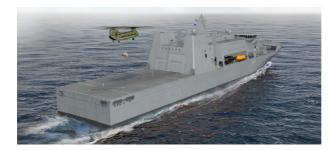
ELLIDA™ is a multi-role logistics ship, designed to provide the capabilities needed in future global operations. It offers the flexibility of a large hull, with internal vehicle and stowage decks, weather deck stowage and additional accommodation.
