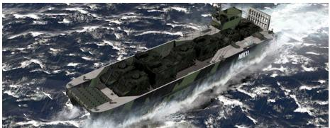
Developed to respond to emerging requirements to distance amphibious forces further from the beach, BMT's CAIMEN®-90 fast landing craft offers huge advances in connector performance. High speeds with exceptional seakeeping, even while carrying a main battle tank, can be realised through BMT's advanced tribow monohull landing craft form.
