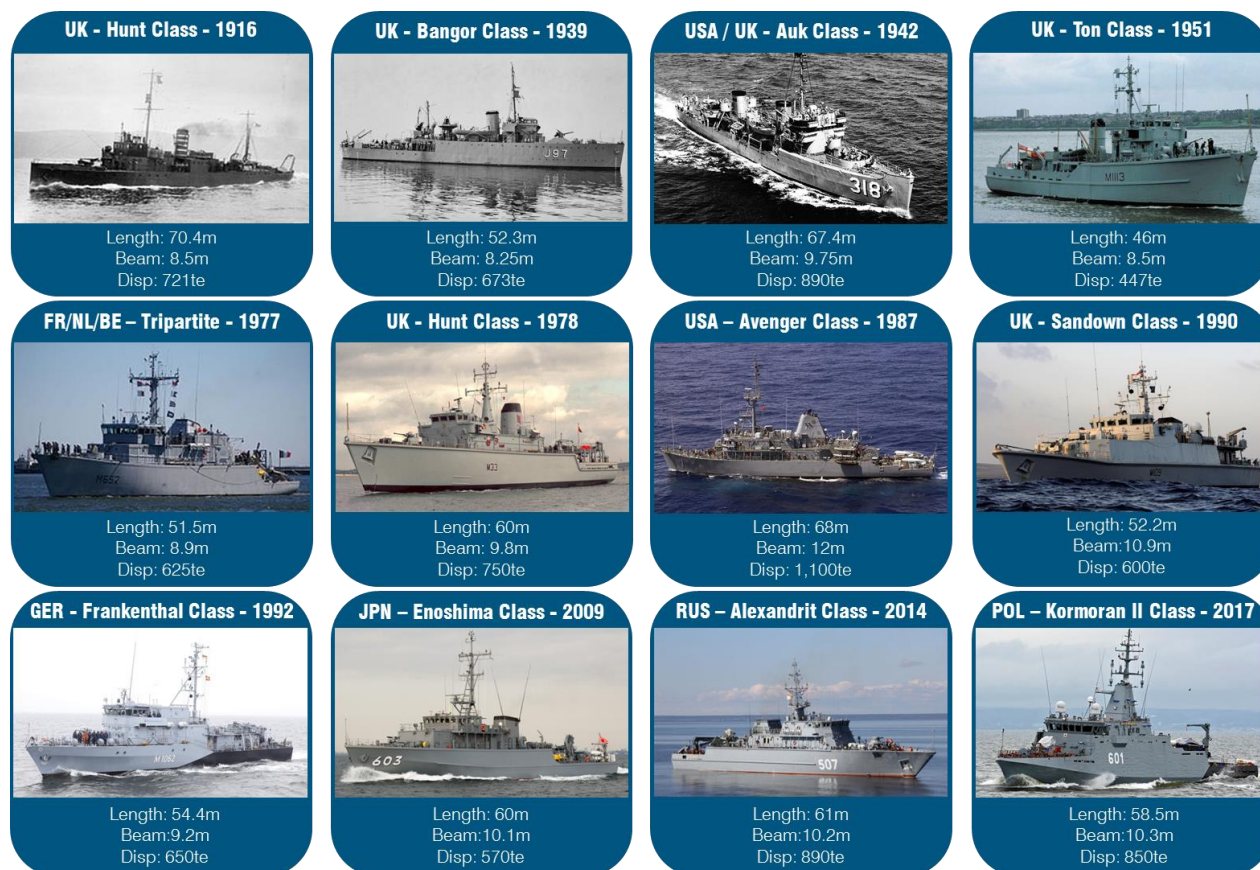
Figure 5 – A selection of Mine Warfare Vessels past and present. These images, and their associated dimensions, show that MCM vessels have not departed far from a common layout and size over the past 100 years. Autonomous technology and developing doctrine is likely to disrupt this trend, leading to a new breed of MCM platform to counter the developing mine threat. (Insert Images from Naval Technology, 2017)
